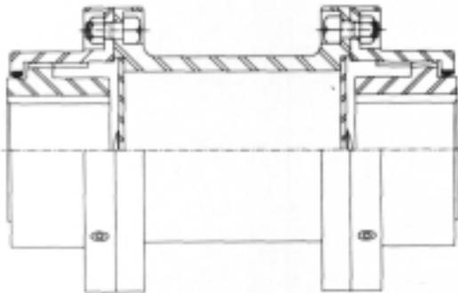
Single engagement styles are normally used in floating shaft assemblies which can be assembled in either rigid flex - flex rigid or flex rigid - rigid flex assemblies (Figure II-A-10).
