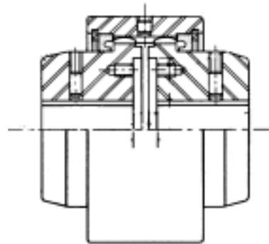
The components of a continuous sleeve coupling are as shown (Figure II-A-8).
