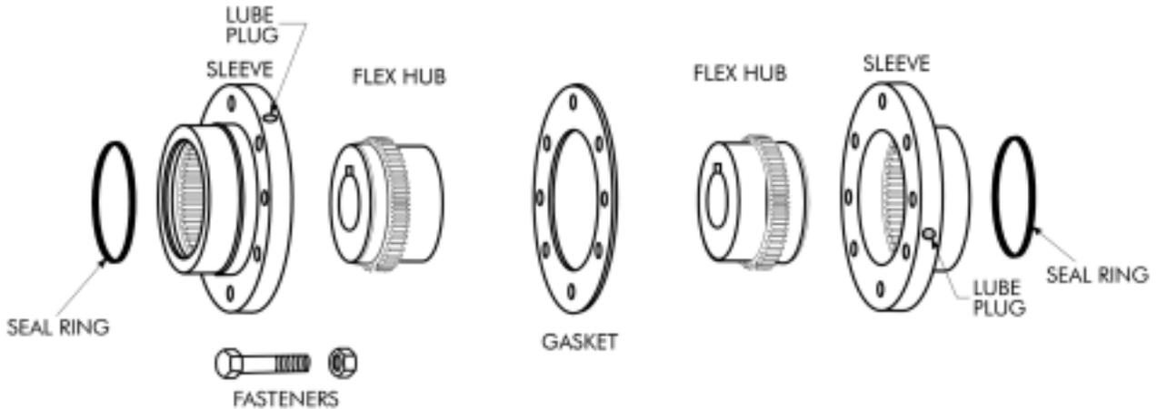
Flanged couplings can be exposed bolt or shrouded bolt types (Figure II-A-6).
