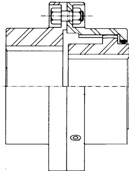
Basically a gear coupling consisting of two contact points is called a double engagement coupling. Alternately, a single engagement coupling has one engagement point and one rigid hub. Components of
