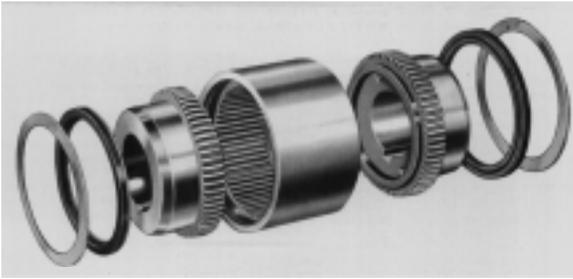
Flanged type gear couplings can be provided with a spacer (Figure II-A-9). This is a configuration commonly used in pump installations to facilitate removal of the pump rotor for maintenance.
