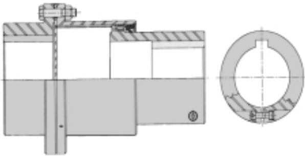
(2) Special hubs and sleeves (Figure II-A-20).
