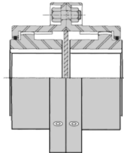
(2) special flanged hubs (Figure II-A-23).
