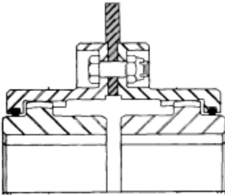
(4) brake wheel (drum) types (Figure II-A-25).
