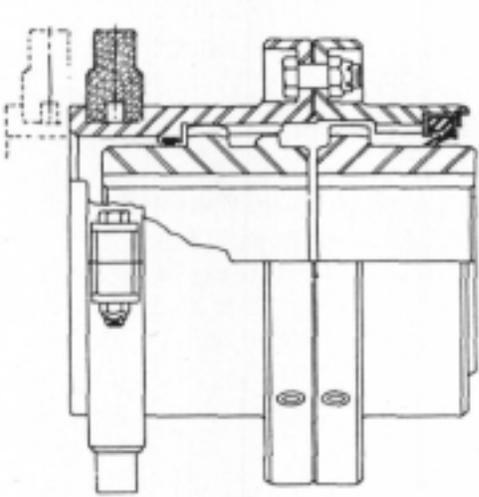
(8) Shear pin coupling(Figure II-A-29)
